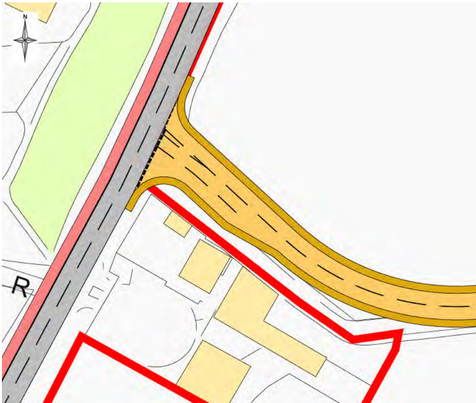
Figure 3.4: Option 2 - Priority Junction Arrangement (North of Jigsaw Ash Tree Farm Day Nursery)
